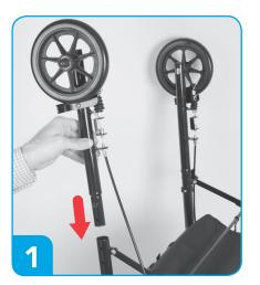
Insert back and front wheels using E-Clip and hand screw to secure them into place.
